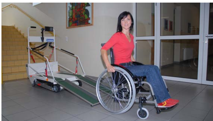
An integrated loading ramp with non-skid surface makes wheelchair boarding easy
